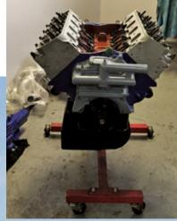
Mat Lagoon from Engine Action in Echuca pulled down the big block Ford motor for inspection. He found a small crack in one of the pistons. A new set of custom made pistons from the US was the solution better to find the problem in Mat's workshop than at 200mph on the salt!
