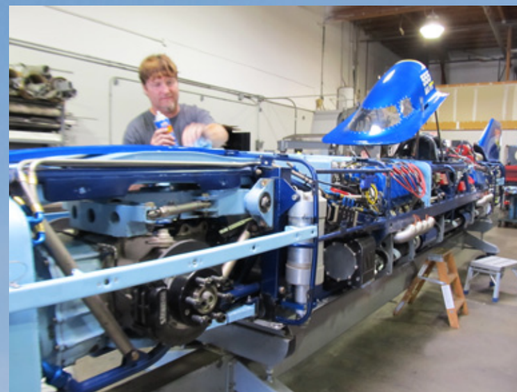
■ Danny's Challenger II rebuild is powered by twin nitro-fueled Hemis
