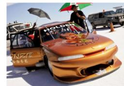
Rod Hadfield's car The Bronze Aussie is getting a nose job. The fibreglass front of the car was creating too much down force and is now being modified to avoid ploughing the salt. The exhaust is being relocated after causing a fire at the last meeting and Rod is still determined to beat John Lynch's 301mph pass. Rod Hadfield is DLRA member #3 and has never missed racing in a DLRA event yet.
