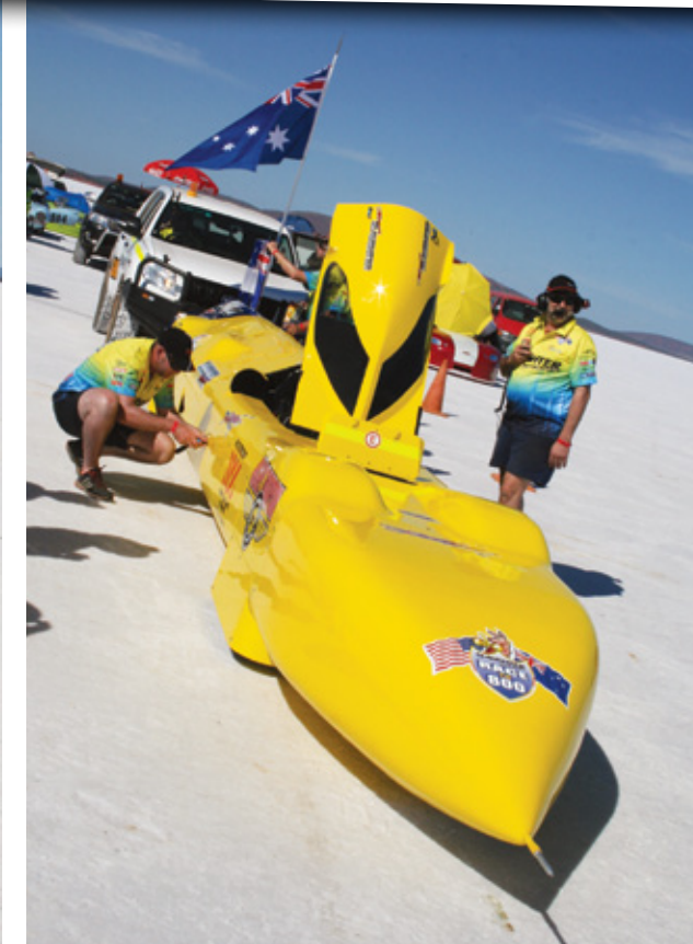
■ The streamliner is 11 metres long and only 800 mm to the top of the body.
